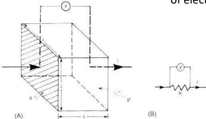
Electrical resistivity (Ohm x m) is a measure of a material's property to oppose the flow of electric current. Its inverse is the electrical conductivity (S/m).
