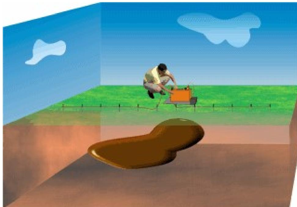
The method of measuring subsurface resistivity involves placing four electrodes in the ground in a line at equal spacing, applying a measured AC current to the outer two electrodes, and measuring the AC voltage between the inner two electrodes. A measured resistance is calculated by dividing the measured voltage by the measured current. This resistance is then multiplied by a geometric factor that includes the spacing between each electrode to determine the apparent resistivity.
