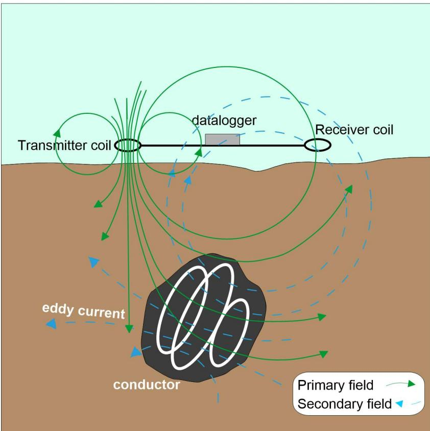
Electromagnetic induction (EMI) is based on the mutual induction among three coils.
